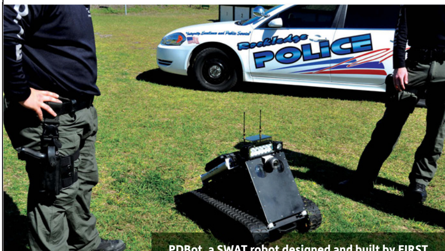
PDBot, a SWAT robot designed and built by FIRST Robotic Competition students from The Pink Team for their local police department.
