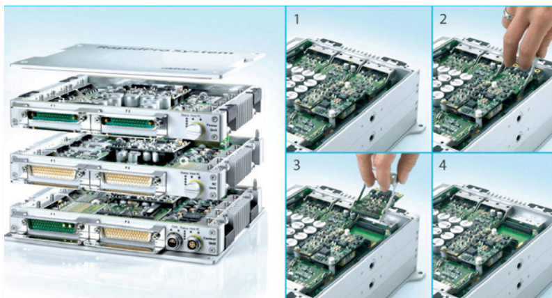
FIGURE 1. Sensors and actuators are adapted for rapid control prototyping with the help of the RapidPro Signal Conditioning Unit and the RapidPro Power Unit. The MicroAutoBox unit is at upper left.
