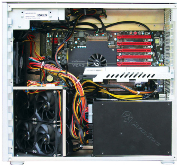
The power supply and fans for the liquid cooling system block access to the CPU and memory sockets. But there's plenty of expansion, thanks to seven PCIe slots.
